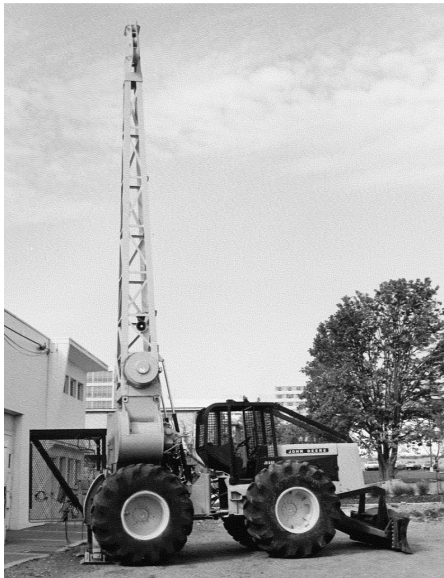
Figure 3: Left- Profile image of original PeeWee yarder (source: USDA Forest Service). Right- Author's conceptual image of PeeWee Jr. yarder with labeled elements A, B, C. A: locations for anchor points or outriggers for stability and increasing load capacity. B: Simplified, carriage-less butt rigging such as a chain sling or grabinski. C: Light loads and higher-gauge wire (e.g. 3/16") may facilitate use of a snatch block for fast setup.
