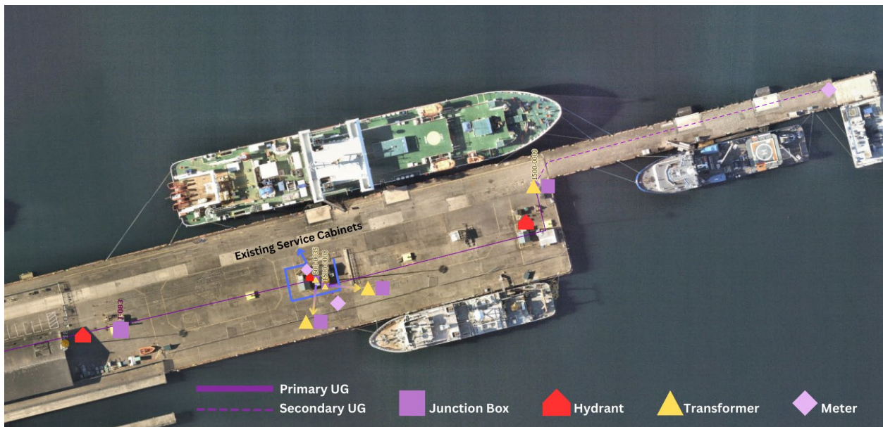
Figure 1. Terminal 1 aerial view with current electrical infrastructure
